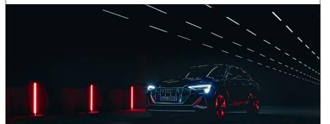
The digital matrix LED headlight can deliver cornering, city and highway lighting as versions of the low-beam light with ultra-high precision. The Audi e-tron Sportback 55 guattro<sup>2</sup> with digital matrix LED headlights is shown above in the Audi light testing tunnel.
